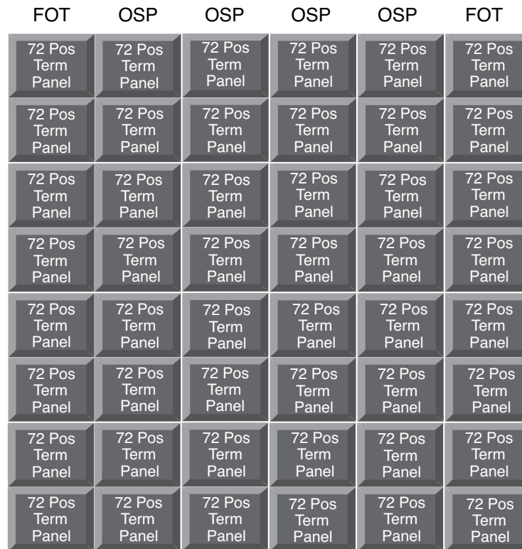
Figure 16. ODF cross-connect configuration with 2:1 OSP:FOT ratio
