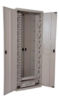
ADC FDF-01 fibre distribution frame provides mounting locations for termination, splice and storage panels. This frame is with front and rear access with lockable doors. The FDF provides vertical slack storage and cable management. This ensures bend radius protection and better fibre management.
