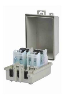
Kronnection Box DT PLUS 2 is used as a line equipment termination point for 2 pairs i.e. for transferring drop wire lines (over head cables) to the telephone cables in the building. Two DT PLUS modules can be mounted in each box to connect 2 solid drop wire lines.
