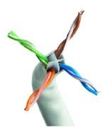
This Category 6, UTP 4 -pair cable is an unscreened cable with PVC outer sheath, for use in high speed data communication. With internationally defined physical and electrical performance up to 250MHz.
