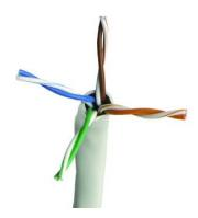
This Category 5e UTP 4-pair CMR Cable is an unscreened cable with PVC outer sheath with rip cord, designed to provide Category 5e Enhanced Link and Channel performance with internationally defined physical and electrical performance up to 100MHz.
