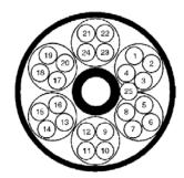
NOTE: The 25th pair is twisted around the filler (Patent #6,259,031)
