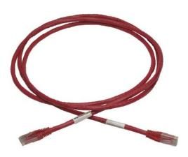
For patching between two RJ45 outlets in a Category 6 network where patching is required between a 568A wired system and a 568B wired system. Each RJ plug has a latch protector to reduce the possibility of snags within the cord bundle.
