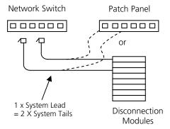
System leads are made from solid conductor materials with an RJ45 plug on each end. Better Insertion Loss than patch cords. Patented impedance matching for zero-bit errors.
