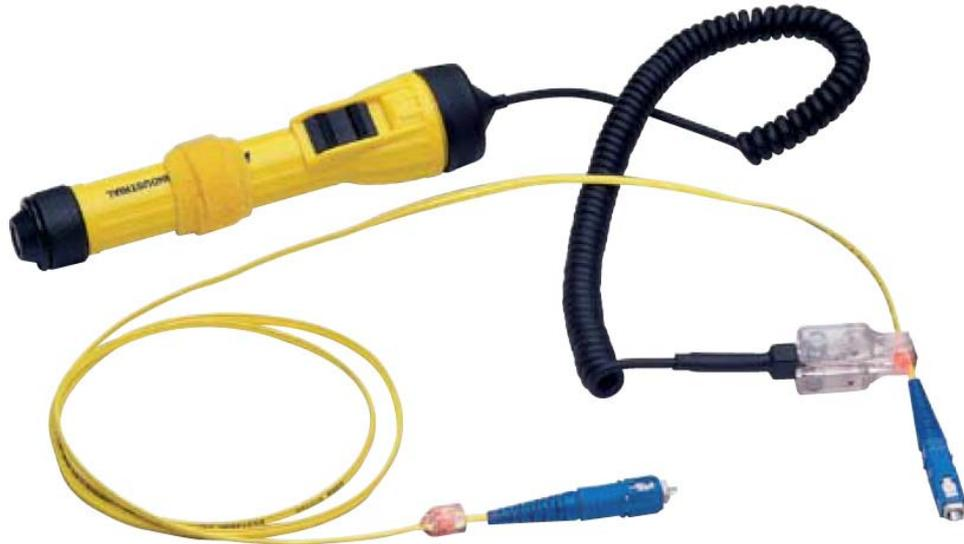
ADC's innovative TracerLight® Connector Identification System offers a quick and accurate method of identifying the termination point of optical patch cords. Each end of a TracerLight® patch cord features a flashing light source allowing technicians to visually trace individual patch cords from one end to the other without pulling or affecting the patch cord.
